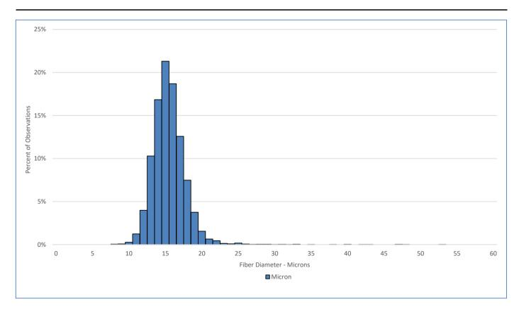
Test Performed According to Method AS/NZS 4492.5:2000
