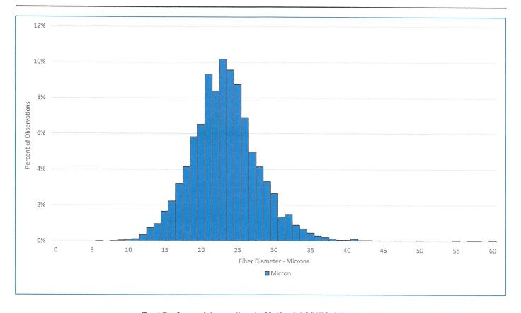
Test Performed According to Method AS/NZS 4492.5:2000
