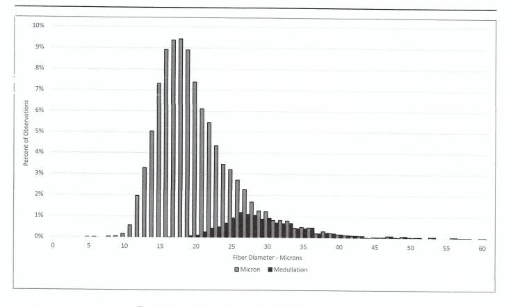
Test Performed According to Method AS/NZS 4492.5:2000
