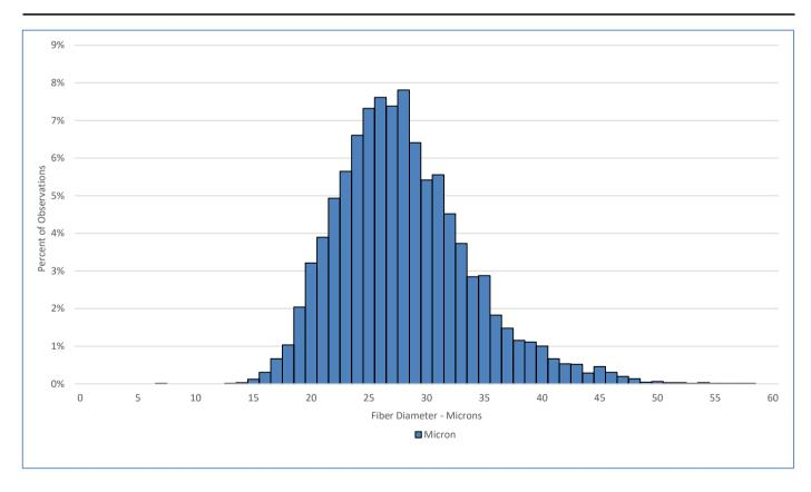
Test Performed According to Method AS/NZS 4492.5:2000
