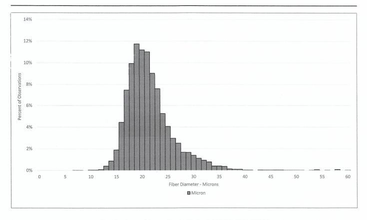
Test Performed According to Method AS/NZS 4492.5:2000
